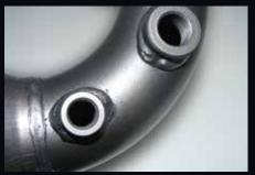
Large diameter turbo dump pipe incorporating EGT (1/4" BSP) & O2 (18mm x 1.5mm Pitch) sensor fittings.
