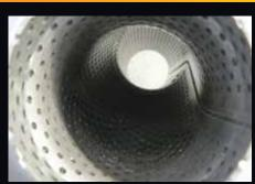
Perforated tube high flow muffler internals supported with a case stiffener.
