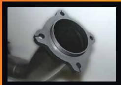
10mm thick 4 bolt pipe through flange design for perfect fitment accuracy.
